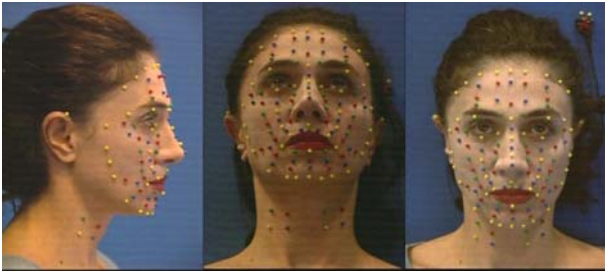
Figure 1. 125 colored beads have been glued on the subject's face along Langer's lines so as to cue geometric deformations caused by main articulatory movements when speaking.
