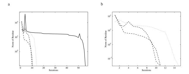
Figure 7: Evolution of residues during optimization; — 1 harmonic, - - 2 harmonics, -.- 3 harmonics, ... 10 harmonics (a) all cases (b) zoom on 2, 3 and 10 harmonics
