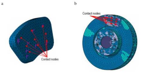
Figure 1: Finite element models of the brake system (a) Pad (b) Disc
