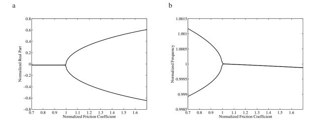
Figure 2: Stability analysis (a) Evolution of the real parts of the stable and unstable modes (b) Coalescence of the two corresponding eigenvalues
