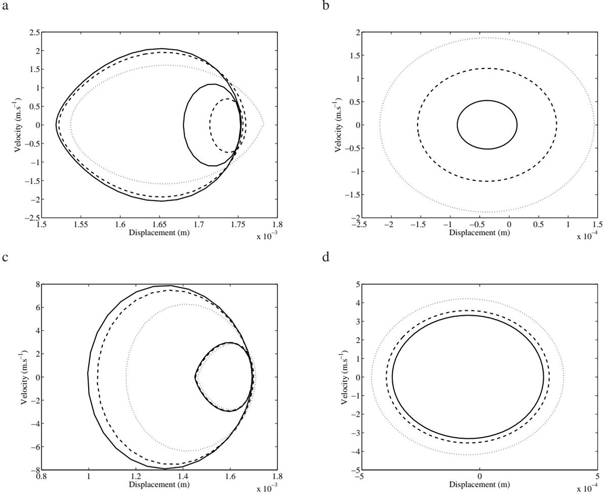
Figure 12: Limit cycles for equally damped modes and plotted for two different  $\mu$  (a-b) Limit cycles plotted at  $\mu = 1.07\mu_0$  — 1<sup>st</sup> case, - - 2<sup>nd</sup> case, ... 3<sup>rd</sup> case (c-d) Limit cycles plotted at  $\mu = 1.4\mu_0$  — 1<sup>st</sup> case, - - 2<sup>nd</sup> case, ... 3<sup>rd</sup> case; (a-c) Pad, (b-d) Disc
