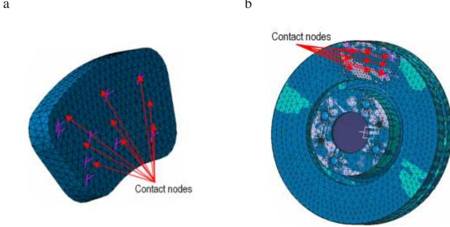
Figure 1: Finite element models of the brake system (a) Pad (b) Disc
