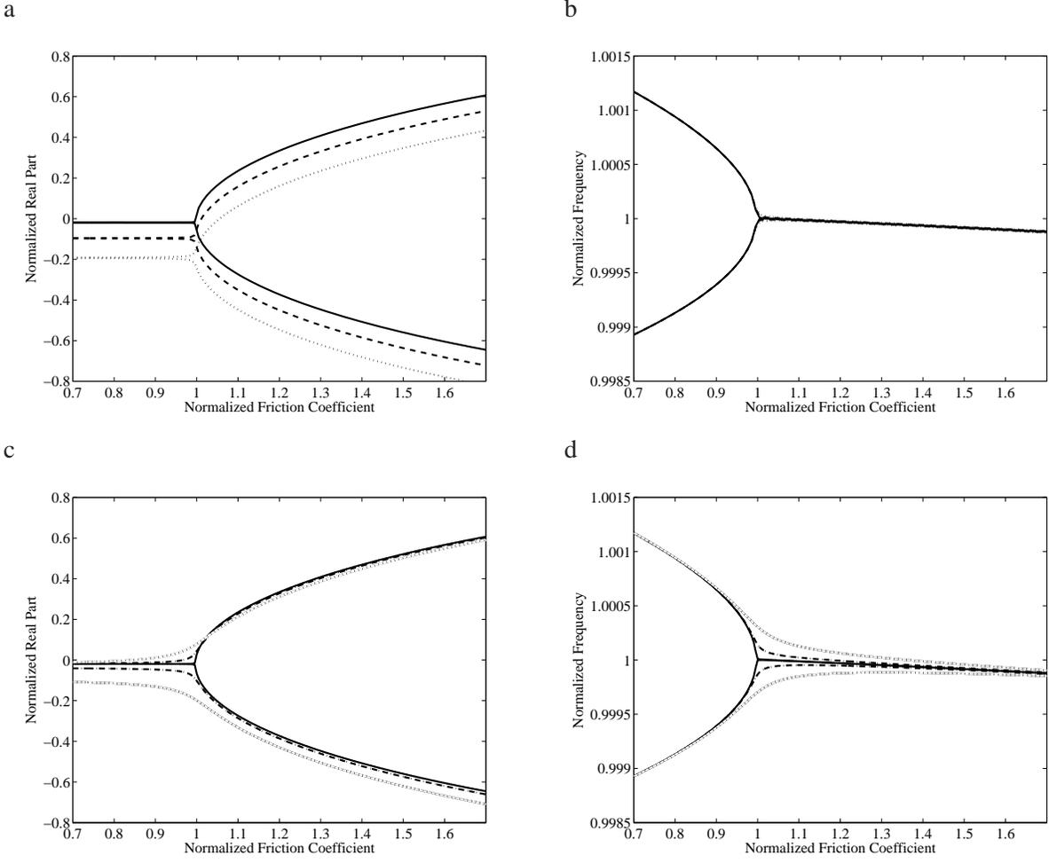
Figure 11: Evolution of real parts and frequency coalescences (a-b) equally damped: — 1<sup>st</sup> case, - - 2<sup>nd</sup> case, ... 3<sup>rd</sup> case (c-d) non-equally damped: — 1<sup>st</sup> case, - - 6<sup>th</sup> case, ... 7<sup>th</sup> case
