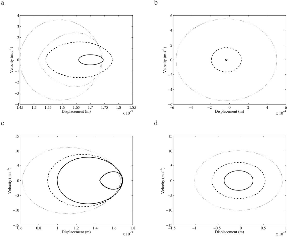
Figure 14: Limit cycles for non-equally damped modes and plotted for two different  $\mu$  (a-b) Limit cycles plotted at  $\mu = \mu_0$  — 1<sup>st</sup> case, - - 6<sup>th</sup> case, ... 7<sup>th</sup> case (c-d) Limit cycles plotted at  $\mu = 1.4\mu_0$ ; — 1<sup>st</sup> case, - - 6<sup>th</sup> case, ... 7<sup>th</sup> case; (a-c) Pad (b-d) Disc
