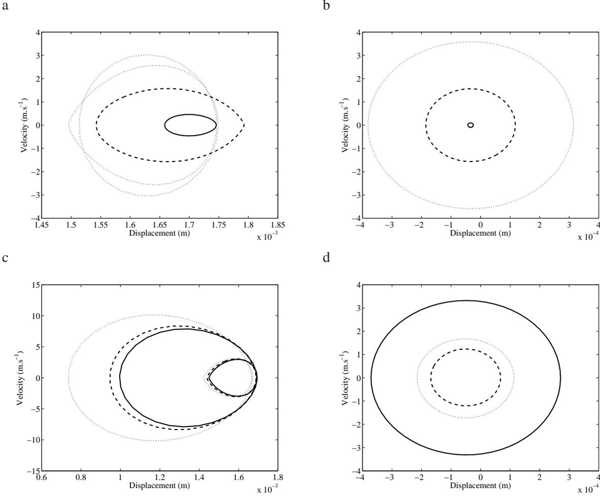
Figure 13: Limit cycles for non-equally damped modes and plotted for two different  $\mu$  (a-b) Limit cycles plotted at  $\mu = \mu_0$  — 1<sup>st</sup> case, - - 4<sup>th</sup> case, ... 5<sup>th</sup> case (c-d) Limit cycles plotted at  $\mu = 1.4\mu_0$  — 1<sup>st</sup> case, - - 4<sup>th</sup> case, ... 5<sup>th</sup> case; (a-c) Pad, (b-d) Disc
