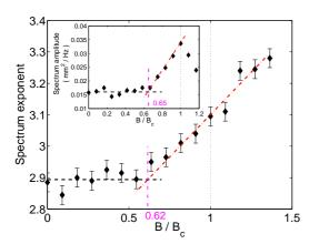
FIG. 3: Exponent of the magneto-capillary spectrum as a function of the dimensionless magnetic induction  $B/B_c$ . Inset: Amplitude of the power spectrum (averaged between 8 and 18 Hz) as a function of  $B/B_c$ . Forcing parameter:  $1 \le f \le 4$  Hz.  $B_c = 294$  G.
