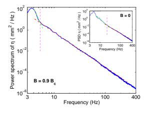
FIG. 2: Power spectrum of  $\eta(t)$  for two values of B. Inset: B = 0: Gravity and capillary wave turbulence regimes. Dashed lines have slopes -4.6 and -2.9. Crossover:  $f_{gc} \simeq 20$  Hz. Main:  $B = 0.9B_c$ : Magneto-capillary wave turbulence. Dashed line has slope -3.3. Crossover:  $f_{gc} \simeq 5$  Hz. Forcing parameters: 1 - 5 Hz.  $B_c = 294$  G.
