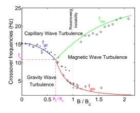
FIG. 4: Rescaled crossover frequencies,  $\bar{f}(B) \equiv f_{gc}(0) \times f(B)/f(0)$  as a function of *B* for different frequency bandwidths of the random forcing: (×) 1 to 4 Hz, ( $\diamond$ ) 1 to 5 Hz, and (+ or  $\circ$ ) 1 to 6 Hz. Theoretical curves  $f_{gc}$ ,  $f_{gm}$  and  $f_{mc}$  are respectively from Eqs. (5), (6) and (7). The triple point ( $f_t = 10.8$  Hz,  $B_t/B_c = 0.65$ ) is from Eq. (8).
