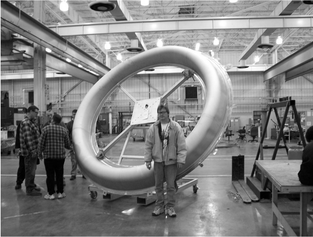
Figure 6. A fully SPF formed 5083-SP jet engine leading edge Nacelle Inlet made by FSW butt welding of four separate segmented blanks prior to forming.
