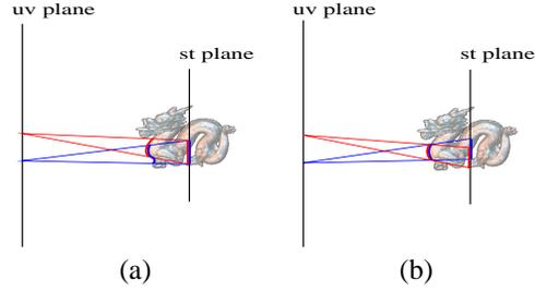
Figure 4: (a) A  $2 \times 2 \times 2 \times 2$  block of *uvst* does not cover the same region of the object; (b) With  $2 \times 2$  blocks of *st* samples, it is possible to associate pixels corresponding to the same region of the object for several viewpoints.
