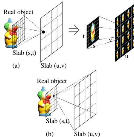
Figure 2: Light field representation. (a) an image corresponds to one  $uv$  sample associated with the whole  $st$  plane; (b) conversely, one  $st$  sample associated with all the  $uv$  directions provides radiance samples passing through the point located in  $(s, t)$ .
