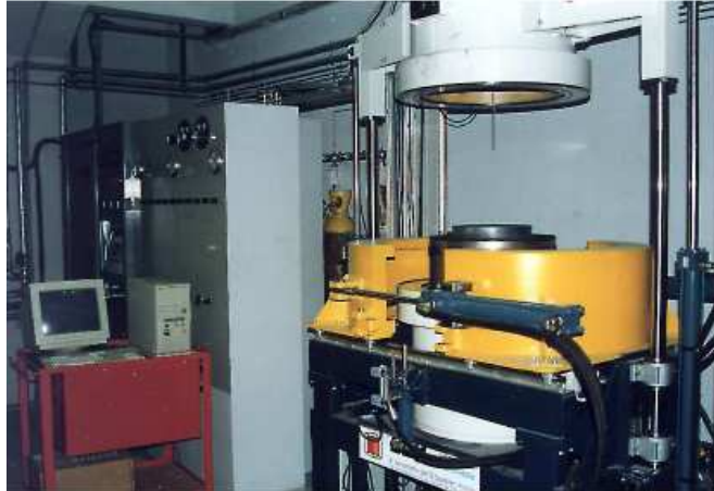
Figure 1: Experimental superplasticity forming machine at ENSAM ANGERS
