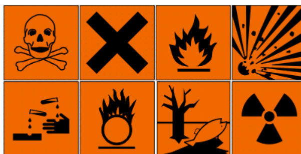
Figure 5: Chemical product security symbols: toxic, irritant, inflammable, explosive, corrosive, oxidant, dangerous for the environment, radioactive
