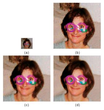
Fig. 12. Using vector-valued regularization PDE' for image magnification ( $\times$ 4). (a) Original color image ( $64 \times 64$ ). (b) Bloc interpolation. (c) Linear interpolation. (d) Interpolation with PDEs.
