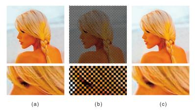
Fig. 11. Using vector-valued regularization PDEs for image reconstruction. (a) Color image, (b) removing 50 percent of the pixels, and (c) reconstructured image.
