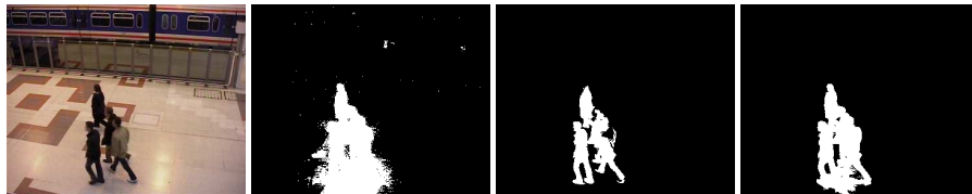
Fig. 2. Background subtraction with illumination changes (PETS 2006 dataset). From left to right respectively, the original image (Frame 165), the segmented image obtained by the MGM, the result obtained using the T2 FMGM-UM and the T2 FMGM-UV
