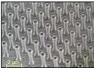
Fig. 5. Foot of Geckoes are composed of hair having spatulas at their tip (100 to 200 nm in diameter) (from (Geim et al. 2003)).
