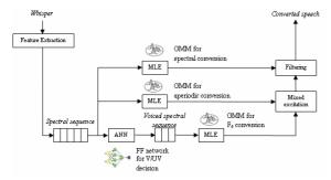
Figure 2: Conversion process of NAM-to-Speech system. Spectral Estimation.
