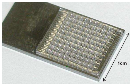
Figure 2: The microfluidic distribution system stuck on an hollowed silicon matrix
