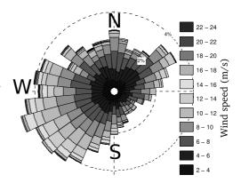
FIG. 2. Wind rose for the years 2006 to 2008 at point A, based on ECMWF analyses. The observations at BEAtrice buoy give a similar result. For each direction, the cumulative frequency is indicated with wind speeds increasing from the center to the outside, with a maximum of 4.3% maximum from West-South-West (heading 250°). An isotropic distribution would have a maximum of 2.7%.
