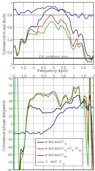
FIG. 4. Rotary co-spectra of the wind and wind stress with the radarderived current, Stokes drift and Eulerian current. (a) magnitude and (b) phase. The number of degrees of freedom is 108 at the spectral resolution of 0.09 cpd. Coherence is significant at the 95% confidence level for a value of 0.1. Negative and positive frequencies are clockwise and counter-clockwise polarized motions, respectively.
