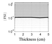
Fig. 5. Evolution of FSI critical value as function of the porous thickness.
