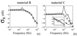
**Fig. 4.** Radiation efficiency simulated with the Biot model (solid line) and the limp model (circles): (a) material B, (b) material C.
