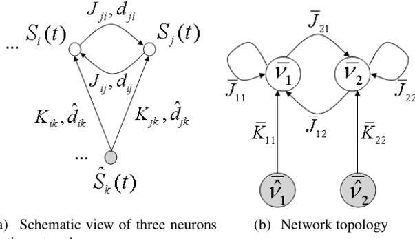
(a) Schematic view of three neurons in the network
