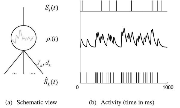
Figure 2. Poisson neuron model. (a) Schematic view of the neuron, with the cell body or soma (circle), the dendritic inputs (below) and the output axon (above). (b) Illustration of the variation of  $\rho_i(t)$  (*middle plot*) for a given succession of pre-synaptic spikes  $\hat{S}_k(t)$  (*bottom spike train*) and the resulting output  $S_i(t)$  (*top spike train*).
