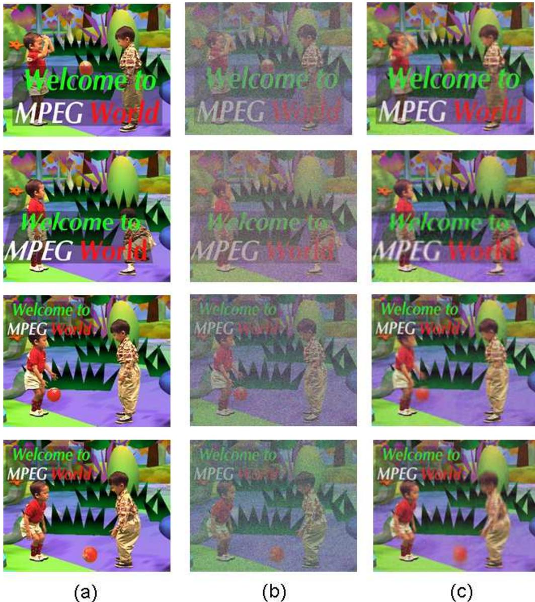
**Figure 6.** Extracting of four images issued: (a) original colour video, (b) noisy colour video and (c) colour video denoised with the 3-D DART in RGB space
