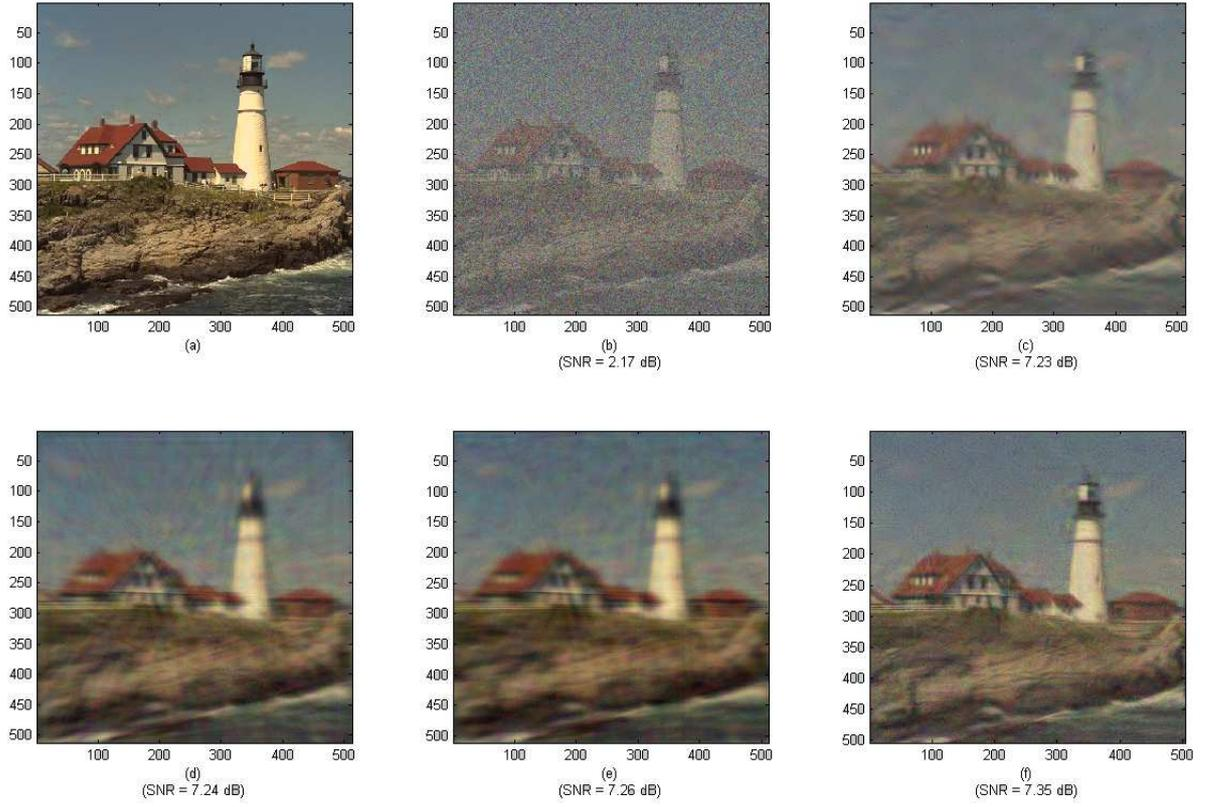
**Figure 4.** (a) Original image (b) Noisy image (c) denoising with the undecimated wavelet transform (d) denoising with the Ridgelet based on the Fast Slant Stack transform and undecimated D20 wavelets (e) denoising with the DART based on Naive lines and undecimated D20 (f) denoising with the local-DART based on Naive lines and undecimated D20 wavelets
