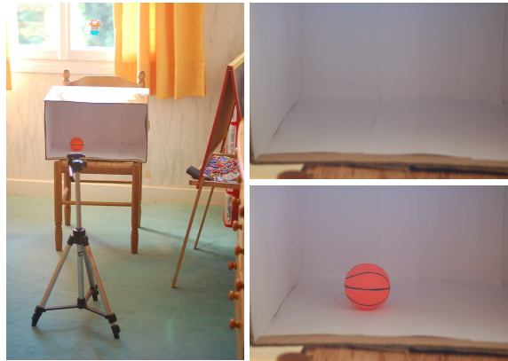
Figure 8: Photographs of indirect shadows: (left) Nicolas bedroom experimentation place; (top-right) photograph with indirect natural lighting without object; (bottom-right) same lighting conditions with an object. Note the shadows on the box floor.
