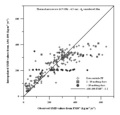
**Fig. 3.** Comparison between observed SMB values from filtered observational SMB data sets (M07) and interpolated SMB values averaged in 100 km resolution (A06-100) with distribution pattern of observed SMB points located in **Percolation Facies** (**PF**~melting events) areas. Cumulative melting days are calculated on the basis of 6.9 GHz microwave penetration depth ( $d_p$ ) of 10 m. SMB values are expressed in kg m<sup>-2</sup> yr<sup>-1</sup> (i.e. mm W.E.).
