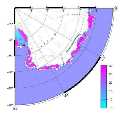
**Fig. 1.** Area of investigation with distribution pattern of surface melting areas observed in 90–180° East Antarctica sector, from 1979 to 2006, by the SMMR (1979–1988) and SSM/I (1988-onward) microwave radiometers. Crosses represent the filtered observed SMB data resulting from M07. Melting areas are expressed in average melting days by year.
