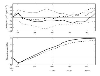
**Fig. 5.** Top panel: Streamline average of the surface density flux (thick line), and the thermal (thin line) and haline (dashed line) contributions. The density flux of the CORE sensitivity experiment is indicated by the heavy dashed line. Bottom panel: streamline-averaged Ekman transport for the reference case (solid line) and the CORE experiment (dashed). The vertical dashed line indicates the southern limit of the ACC belt.
