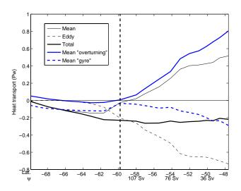
**Fig. 13.** Meridional depth-integrated heat transport across streamlines for the reference experiment. The total and eddy part correspond to the numbers in Table 2 for the north and south boundary of the ACC region (this south boundary is marked by a vertical black line). The time-mean heat transport (thin black line) is further decomposed into two terms, the "overturning" and "gyre" parts.
