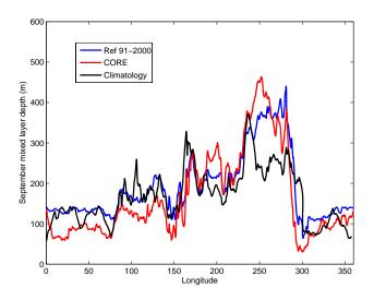
**Fig. 7.** Average mixed layer depth for the month of september, in the model and in the climatology of de Boyer Montégut et al. (2007), estimated with a density criterion. The model mixed layer depth is estimated as the depth were density is  $0.1 \, \mathrm{kg \, m^{-3}}$  larger than at the surface.
