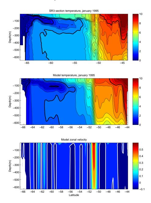
**Fig. 3.** Observations and model results along the WOCE SR3 section. Top panel: observed potential temperature (January 1995). Temperatures of 0, 2 and 10°C are indicated in bold. Middle panel: model potential temperature averaged for January 1995. Bottom panel: zonal velocities (m/s). The zero contour is underlined in white.
