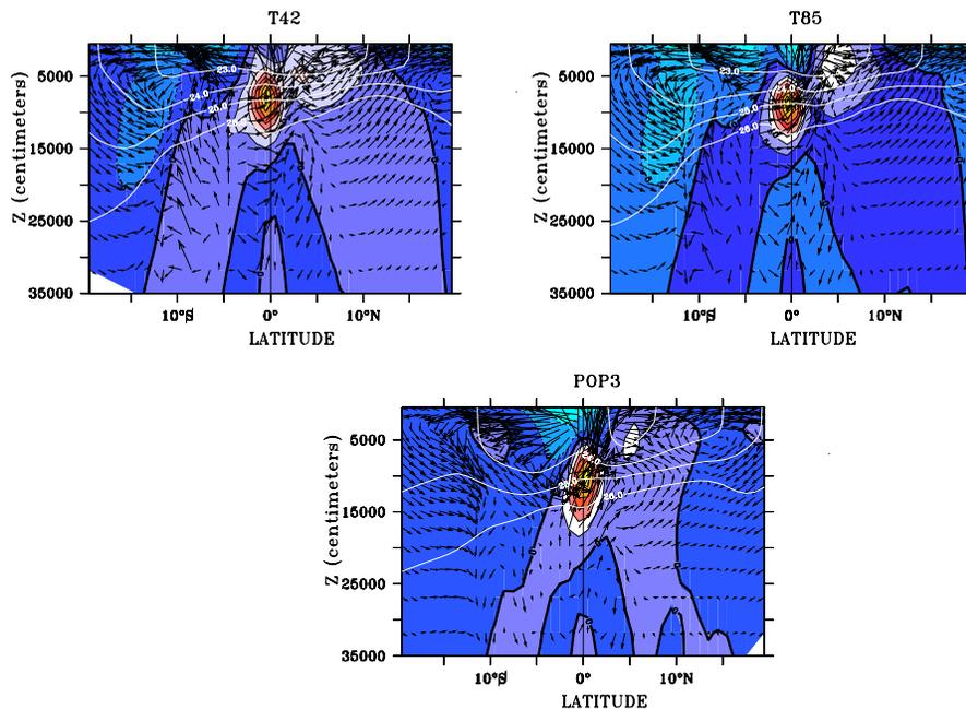
**Fig. 1.** mean meridional versus vertical velocity ( $\times 10^3$ ) circulation vectors superimposed on the zonal velocity field (contour interval is 5 cm/s for T85 and T42 – upper panels, and 10 cm/s for POP3 – bottom panel). Thick white horizontal curves are selected isopycnals at 5 kg m<sup>-3</sup> contour intervals. Note that for each run a different isopycnal surface crosses the core of the EUC. Thick black line is the zero contour for zonal velocity (in color shading).
