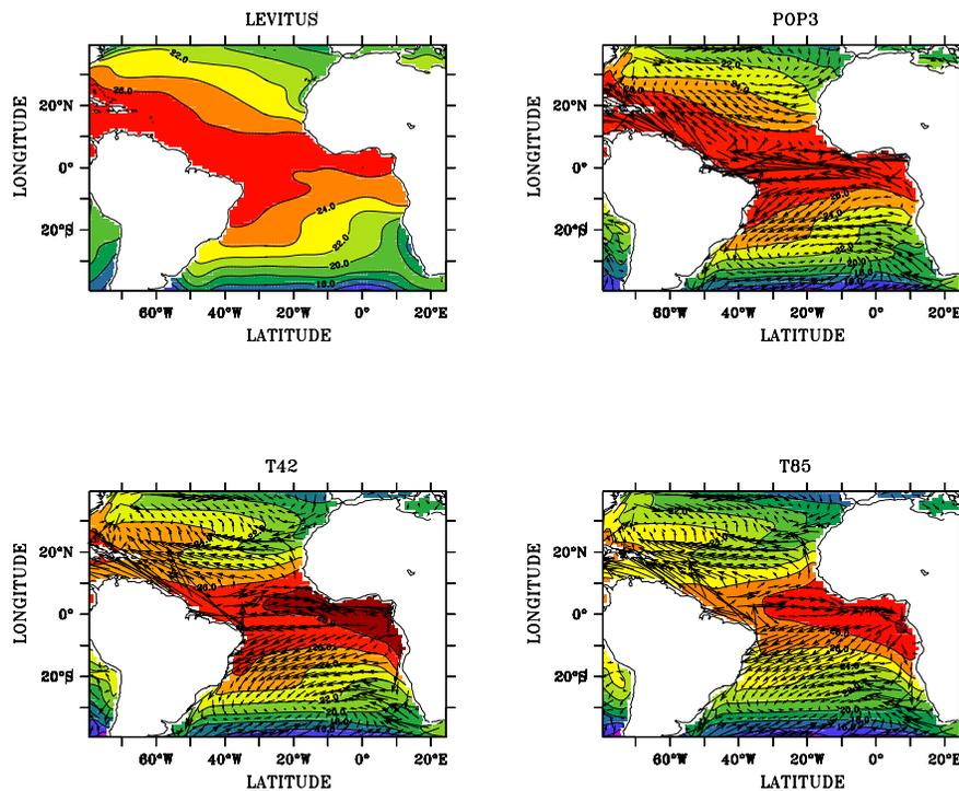
**Fig. 3.** Climatological mean (Levitus et al., 2000), model surface temperature (contour interval is  $2^{\circ}\text{C}$ ) and current field vectors (cm/s).
