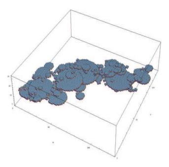
**Fig. 8c.** The percolating cluster from the realization shown in Fig. 8b. Although only a relatively thin layer of disks participate in the percolating cluster, the possibility of connecting in the vertical direction is enough to reduce the bubble percolation threshold  $P_c$  well below the 2-D value  $\approx 0.6$  (which we would obtain in the limit of planar disks infinitely thin in the z-direction).
