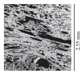
**Fig. 7.** Here is an example of a natural pumice displaying elongated large bubbles compared to less elongated smaller ones (from Santorini volcano). The image is a scanning electronic backscattered image. This image represents a Santorini volcano pumice.
