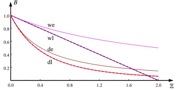
**Fig. 6.** The dependence of the dispersion parameter  $B$  of Eq. (71) and Table 3 for channels of linearly decreasing depth ( $dl$ ), exponentially decreasing depth ( $de$ ), linearly decreasing width ( $wl$ ) and exponentially decreasing width ( $we$ ).
