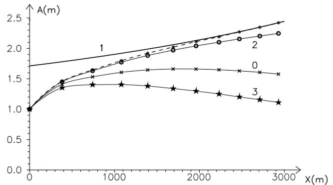
**Fig. 11.** Maximum amplitude of a step-wise perturbation in the process of its disintegration into solitons. The solid line 1 depicts the theoretical prediction of soliton amplitude dependence on distance when dissipation is neglected. The different numerical calculations shown correspond to no dissipation (\*), Rayleigh dissipation ( $\times$ ), Chezy dissipation ( $\star$ ) and Reynolds dissipation ( $\diamond$ ).
