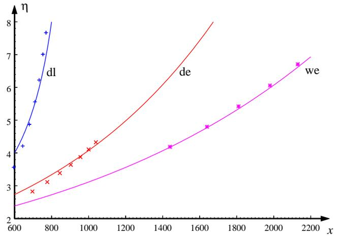
**Fig. 9.** The leading pulse amplitude shown in Fig. 8 as a function of  $x$  computed numerically (symbols) for a channel of linearly decreasing depth (*dl*), exponentially decreasing depth (*de*) and exponentially decreasing width (*we*). The corresponding Green's laws (22) are given for each case in solid lines.
