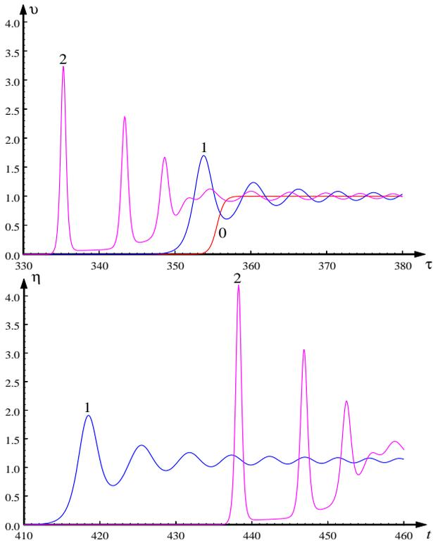
**Fig. 7.** Bore decomposition into solitons for a channel of linearly decreasing depth. The top panel shows time dependence of the solution  $v(\xi, \tau)$  in the reduced coordinates for the initial condition  $\xi = 0$  (curve 0),  $\xi = 18$  (curve 1) and  $\xi = 30$  (curve 2). The bottom panel shows the corresponding perturbation of water surface in the laboratory frame  $\eta(x, t)$  for the last two values of  $\xi$ ,  $x = 532$  m ( $\xi = 18$ ) and  $x = 644$  m ( $\xi = 30$ ).
