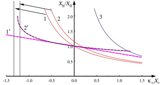
**Fig. 5.** Dependencies of the normalized breaking distances of a Riemann wave,  $X_b/X_0$ , on the normalized gradients of channel depth  $\kappa_h X_0$  (line 1) and channel width  $\kappa_l X_0$  (line 1'). Curve 3 depicts the normalized distance to the channel origin,  $X_{or}/X_0$ , where its depth or width turns to zero according to the linear models (31), (35). Lines 2 and 2' show the influence of the Rayleigh dissipation on wave breaking (see Sect. 3.3.1).
