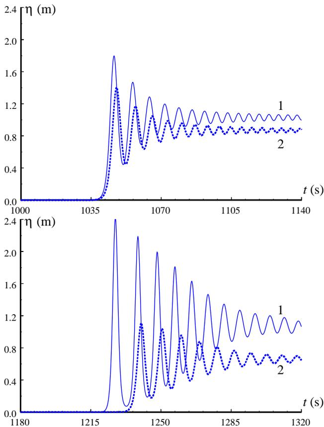
**Fig. 10.** Bore disintegration into solitons without dissipation (curves 1) and with Chezy dissipation (curves 2). The top panel corresponds to  $x = 1080$  m, while the bottom one is for  $x = 2930$  m.
