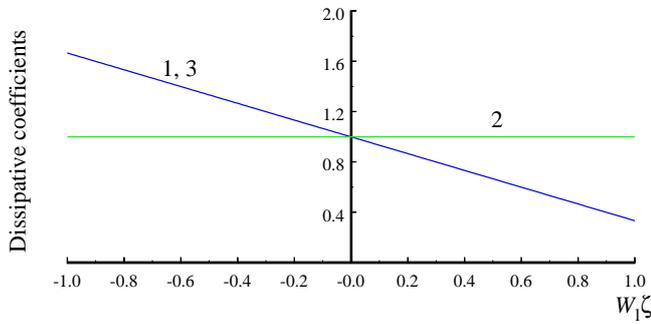
**Fig. 3.** Dependences of the normalized dissipative coefficients  $g_0^l(\zeta)$ ,  $g_c^l$  and  $g_2^l(\zeta)$  labeled respectively 1,2 and 3, on the normalized distance  $W_l \zeta$  for a channel of variable width.
