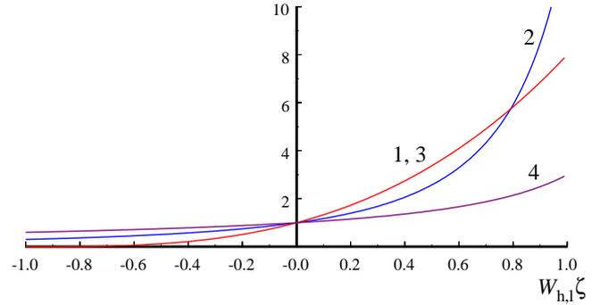
**Fig. 4.** The ratio of the Reynolds dissipation to the Rayleigh one normalized to  $U/h_0$  versus the dimensionless distance  $W_{h,l} \zeta$  for a KdV soliton propagating in a channel of linearly varying depth (curve 1) and width (curve 2) and analogous dependencies for the normalized Ursell parameters (34) (curve 3) and (38) (curve 4).
