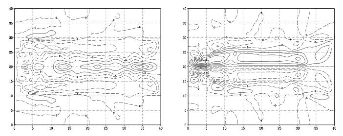
Fig. 5. (a) The "most dangerous" forcing perturbation. (First singular vector of  $H^{(1)}$  matrix.) This perturbation results in  $\delta \|\overline{\omega}\| = 4.15 \times 10^8 \delta \|f\|$ . (b) "Less dangerous" forcing perturbation. (Third singular vector of  $H^{(1)}$  matrix.) This perturbation results in  $\delta \|\overline{\omega}\| = 1.14 \times 10^7 \delta \|f\|$ .
