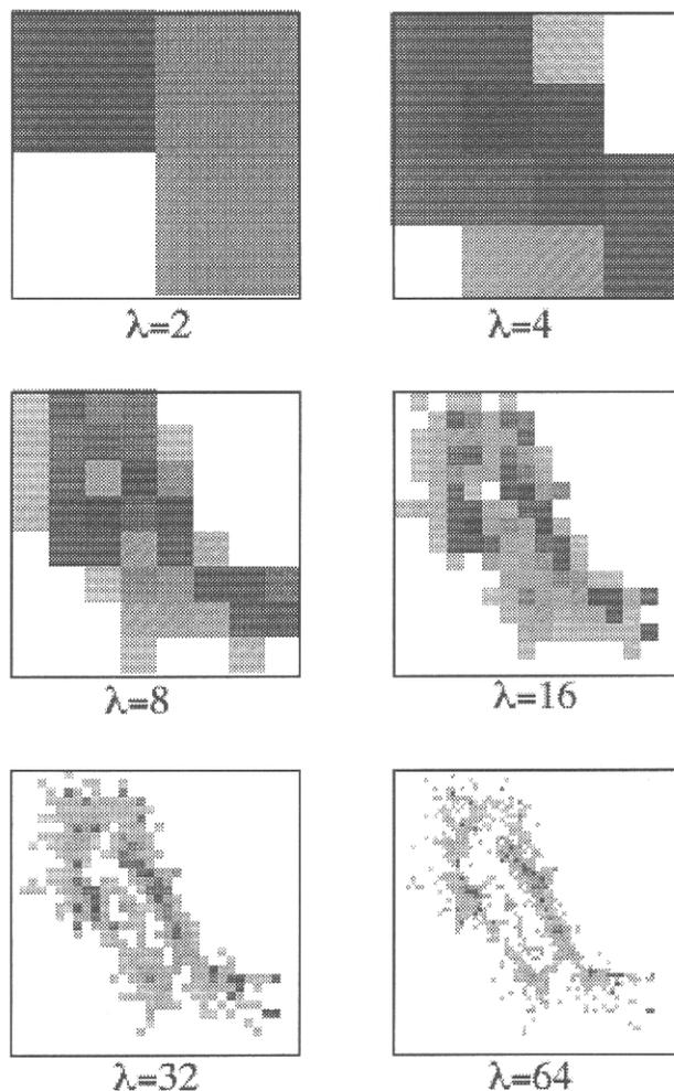
Fig. 1. The seismic field for various values of the parameter  $\lambda$  with  $\eta = 1$ . This figure shows how the picture changes with resolution (*i.e.*  $\lambda$ ).
