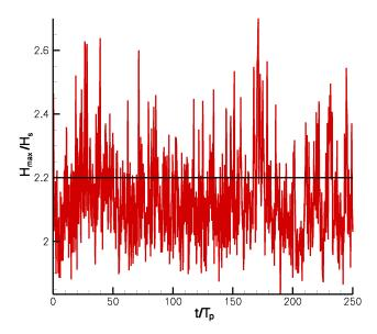
**Fig. 11.** Evolution of  $H_{\text{max}} / H_s$  during time of simulation, directionality n=2.
