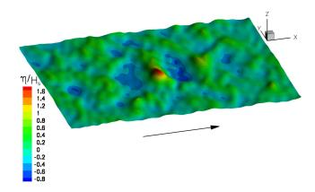
**Fig. 13.** Zoom on the 3-D extreme event  $t=26.5 T_p$ ,  $H_{\text{max}}=2.44 H_s$ .
