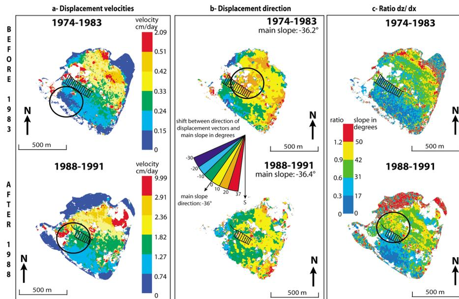
**Fig. 9.** Spatial and temporal evolution of the slip surface geometry of the main body of the la Clapière landslide – the location of the Iglère bar appears in black on each image. Black circles focus on interesting areas. **(a)** Distribution of velocity of total displacements before 1983 and after 1988. **(b)** Distribution of direction of displacements before 1983 and after 1988. **(c)** Distribution of ratio vertical displacements to horizontal ones before 1983 and after 1988.
