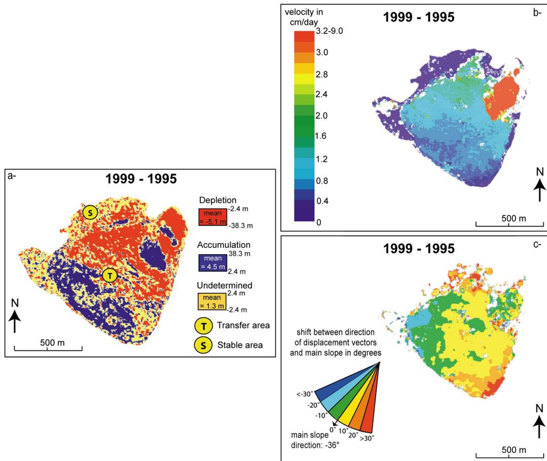
**Fig. 4.** Surface data extracted from DEMs and orthoimages of the la Clapière landslide: (a) differential DEM represented by a three colors map for the time interval 1995–1999, (b) map of displacement velocities for the time interval 1995–1999, (c) map of displacement directions for the time interval 1995–1999.
