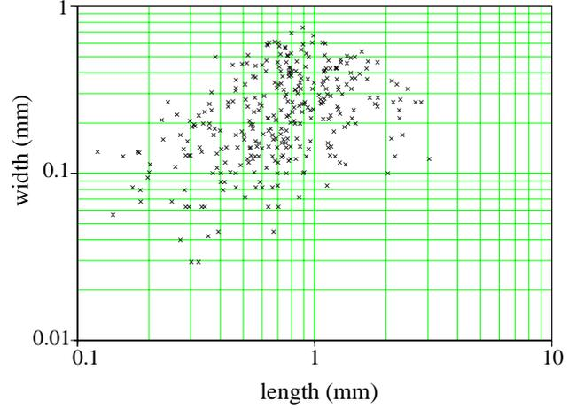
**Fig. 2.** Distribution in size of 300 sawdust particles.
