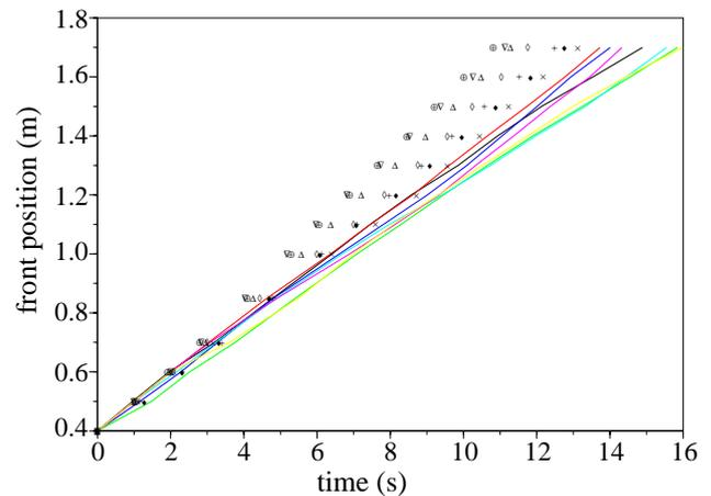
**Fig. 5.** Position of the front as a function of time. The channel inclination is  $45^\circ$ . Points correspond to experimental data with particle entrainment, the solid lines represent the experimental curves without entrainment.
