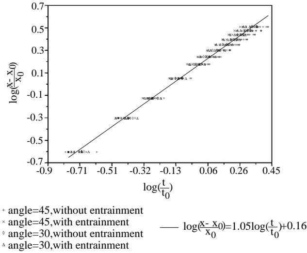
**Fig. 6.**  $\log\left(\frac{x-x_0}{x_0}\right)$  is plotted versus  $\log\left(\frac{t}{t_0}\right)$ , for the four types of experiment we performed. The linear regression obtained from all the points is also plotted.
