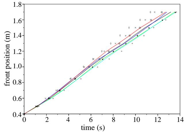
**Fig. 4.** Position of the front as a function of time. The channel inclination is  $30^\circ$ . Points correspond to experimental data with particle entrainment, the solid lines represent the experimental curves without entrainment.
