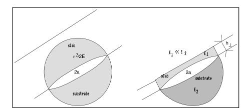
**Fig. 1.** Schematic spatial distribution of stored elastic energy around a basal crack: (a) in the case of a deep slab, and (b) in the case of a shallow slab of depth h
