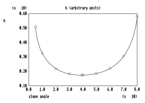
Fig. 2. Variations with slope of the critical slab depth h for avalanche release in the limiting case of a soft shallow slab.
