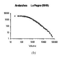
**Fig. 3.** Distribution of avalanche frequency vs. duration of the associated acoustic emission from Val Frejus data (a) or vs. avalanche size (slab depth *x* crown crack length) from La Plagne data (b): the data obey a power law up to a cutoff associated with the spatial scale of the system.
