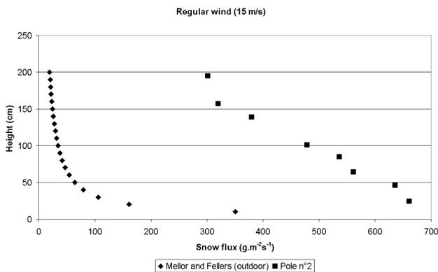
**Fig. 14.** Mean snow flux as a function of height during the experiment.
