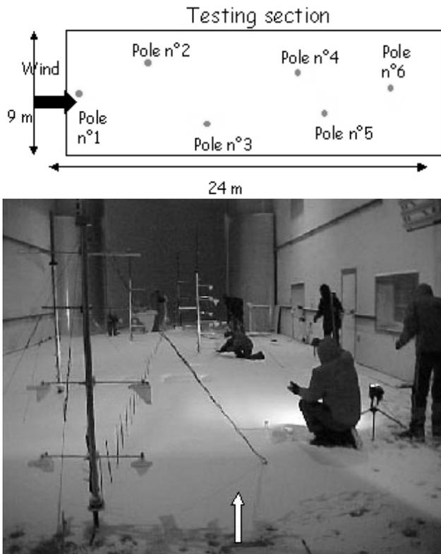
Fig. 2. Experimental set-up in the testing section.
