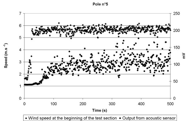
**Fig. 8.** Snow in the recirculation zone: the time to obtain steady-state blowing snow is shorter.
