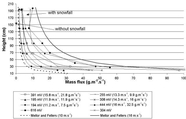
**Fig. 6.** Mean snow flux as a function of height for different natural drifting snow events at Lac Blanc Pass.
