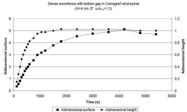
**Fig. 20.** Dimensionless maximum depth and dimensionless area as a function of time for a sand drift generated by a dense snow fence (40 mm) with a bottom gap (8 mm) in the Cemagref wind-tunnel ( $u_*/u_{*t} = 1.3$ ).
