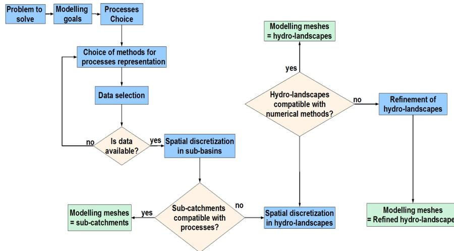
Fig. 1. Flow diagram of the three-level discretization procedure.
