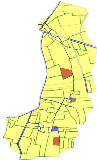
**Fig. 17.** Geometry used in the modelling of the La Fontaine du Theil catchment. Orange fields are drained fields, yellow fields are agricultural fields, green lines are hedges and blue lines are river reaches.
