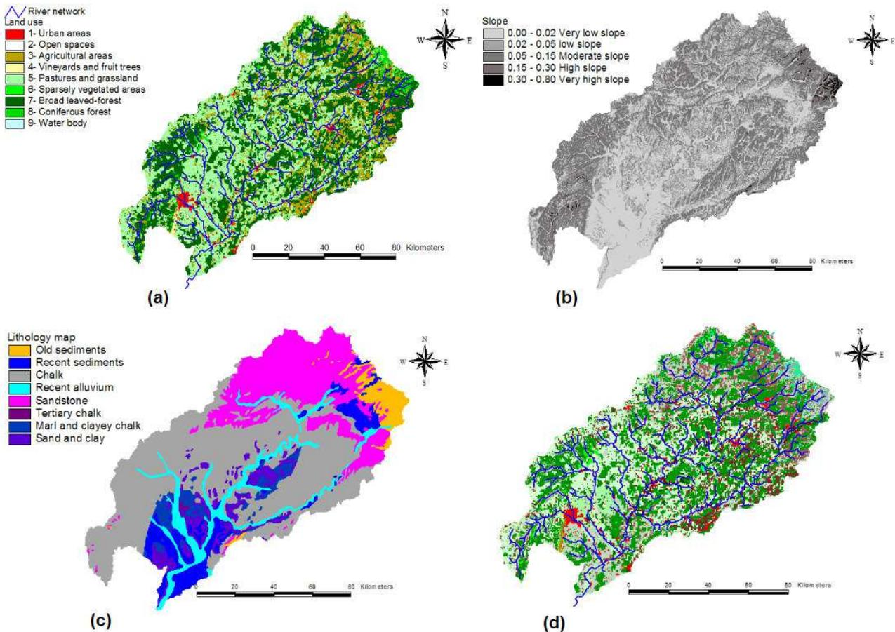
**Fig. 7.** Maps of (a) land-use, (b) slope and (c) lithology on the upper Saône catchment. (d) Map of the combination of the three previous factors. Superimposed is the discretization of the catchments into sub-catchments at the two Strahler order.
