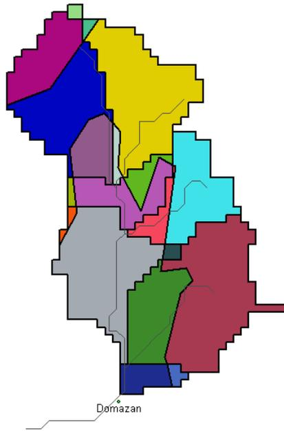
**Fig. 16.** Geometry used in the modelling of a 6 km<sup>2</sup> sub-catchment in the Cévennes-Vivarais region. Colours correspond to the pedolandscape of the soil map, black contour lines correspond to the sub-catchment boundaries and blue lines to the river reaches.
