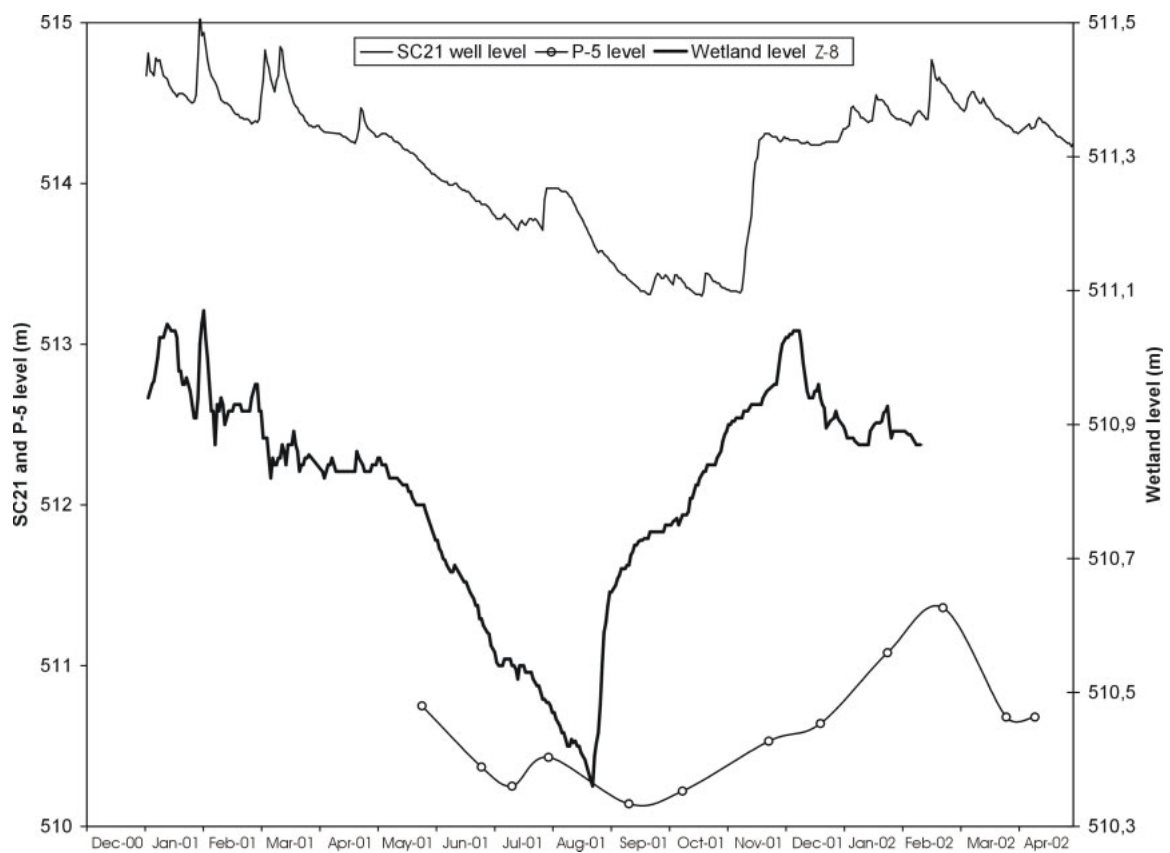
Fig. 6. Groundwater level in the Arkaute well (SC21), a wetland piezometer (P-5) and water level of the outlet of the wetland (Z-8) as function of time.
