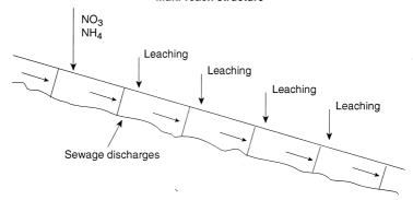
Fig. 3. The structure of the in-stream component of the new version of INCA. (After Whitehead et al., 1998a: published with permission of STOTEN, Elsevier).
