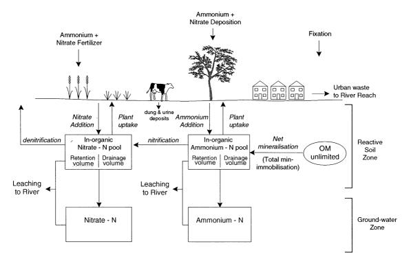
Fig. 2. The structure of the land component of the new version of INCA.
