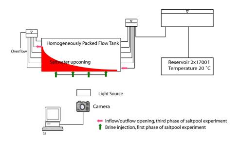
Fig. 1. Schematic experimental setup.
