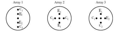
**Fig. 12.** Evaluated sets of electrode arrays.
