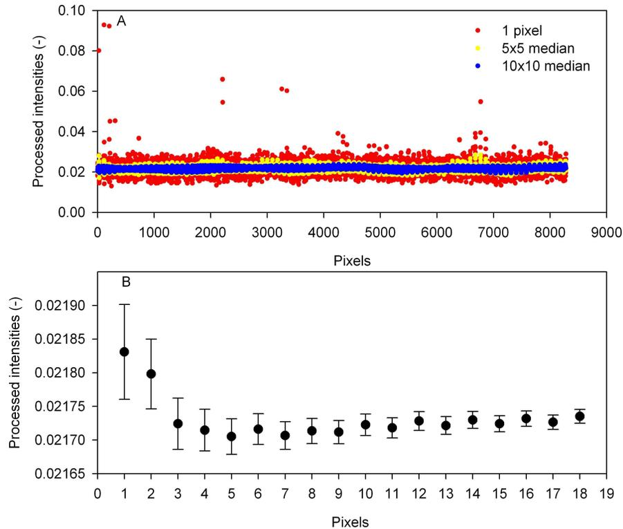
**Fig. 4.** A: Intensities of the 8281 pixels of a square of  $5\text{ cm}^2$  of calibration image  $100\text{ g/l}$  derived as median of squares of 1, 5 and 10 pixels edge length; B: Median of squares of  $1 \times 1$  to  $18 \times 18$  pixels and 95% confidential interval.
