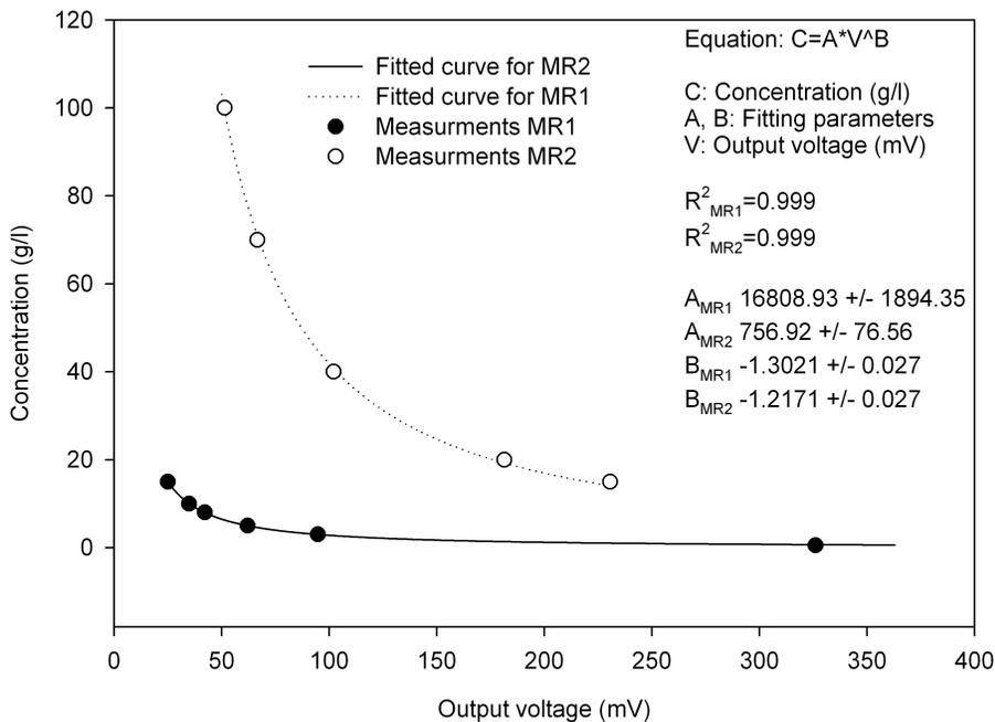
Fig. 14. Calibration curves for the RMC at P2.
