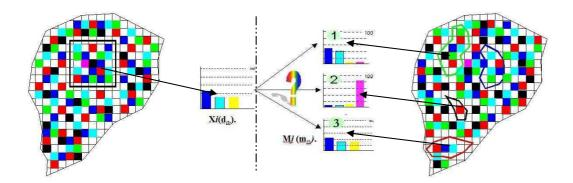
**Fig. 2.** Basic principles for the mapping by landscape classification. On the left map is figured a point to be mapped (the black one) with a squared neighbourhood window and the composition histogram within this window. On the right map are shown the reference zones and their composition histograms. In the middle the Manhattan distance is used to search for the minimum distance between the left histogram and those of the reference zones.
