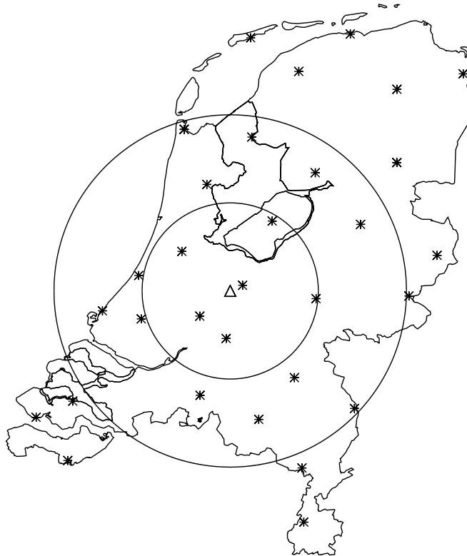
Fig. 9. The locations of the KNMI radar site ( \Delta ) and the automatic KNMI rain gauges ( * ) in The Netherlands. Concentric circles around the radar antenna with a radius of 50 and 100 km give an indication of the distance of the gauges to the radar site.
