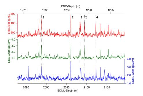
**Fig. 1.** Illustration of a volcanic match based on electrolytical conductivity (Cond) for EDML and  $SO_4$  concentrations or Cond for EDC. The section shown is from a depth range where peak diffusion is already noticeable at EDML. The matches are indicated as vertical dashed lines. Numbers given at each match refer to the confidence value attributed to the matches ranging from "1" ("certain") to "4" ("tentative"). The section shown covers the time from  $\sim$ 90.1 to  $\sim$ 92.6 ka BP.
