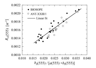
**Fig. 8.** Relationship between remote-sensing reflectance,  $R_{rs}(555)$ , and the ratio of absorption to the sum of absorption and backscattering coefficients,  $b_b(555)/[a(555)+b_b(555)]$ . The data points for the BIOSOPE and ANT-XXIII/1 cruises and the linear function fit to all data are shown. The equation of the fit is:  $R_{rs}(555)=0.03771$   $b_b(555)/[a(555)+b_b(555)]+7.04\times10^{-4}$  (coefficient of determination  $R^2=0.822$ , number of observations N=41).
