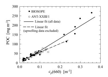
**Fig. 6.** Relationship between surface concentration of particulate organic carbon, POC, and particulate beam attenuation coefficient,  $c_p(660)$ . The data points for the BIOSOPE and ANT-XXIII/1 cruises and the linear function fits to all data (solid line) and the limited data sets with Chilean upwelling stations excluded (dashed line) are shown (see Table 4 for regression coefficients and error statistics).
