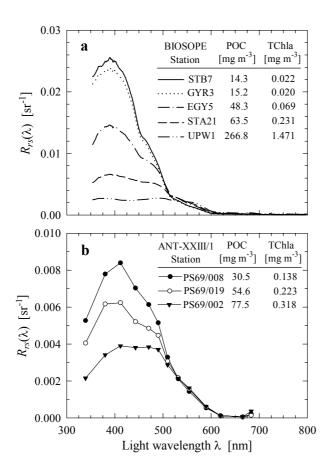
**Fig. 3.** Example spectra of remote-sensing reflectance,  $R_{rs}(\lambda)$ , measured on the BIOSOPE (panel **a**) and ANT-XXIII/1 (panel **b**) cruises at stations with different levels of surface particulate organic carbon (POC) and chlorophyll a (TChla) concentrations. The name of the station and the POC and TChla concentrations are indicated.
