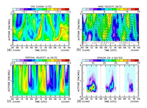
**Fig. 8.** Height-time cross sections of the structure constant  $Cn^2$  (m<sup>-2/3</sup>) (a), horizontal wind (m s<sup>-1</sup>) (b), vertical velocity (m s<sup>-1</sup>) (c) and dissipation rate of turbulent kinetic energy ( $10^{-4}$  m<sup>2</sup> s<sup>-3</sup>) measured with the UHF wind profiler in Saint Chamas during the Mistral episode (J21 to J23). The red solid line in panel (a) represents the ABL top height.
