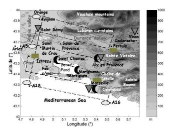
**Fig. 1.** Map of the various instrumented sites and horizontal track of the flights performed by the aircraft during the ESCOMPTE field experiment. Ellipses represent aircraft sounding locations. Triangles indicate radio-sounding sites and black half-moons correspond to the location of UHF wind profilers. Grey rectangles indicate the surface flux stations. Names of town, mountains and valleys are written in black, white and grey, respectively.
