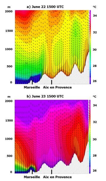
**Fig. 9.** Vertical section of potential temperature (color scale) and horizontal wind simulated by Meso-NH along an axis Marseille-Aix en Provence on 22 June at 15:00 UTC (a) and on 23 June at 15:00 UTC (b). The location of the cross section is shown in Fig. 16b.
