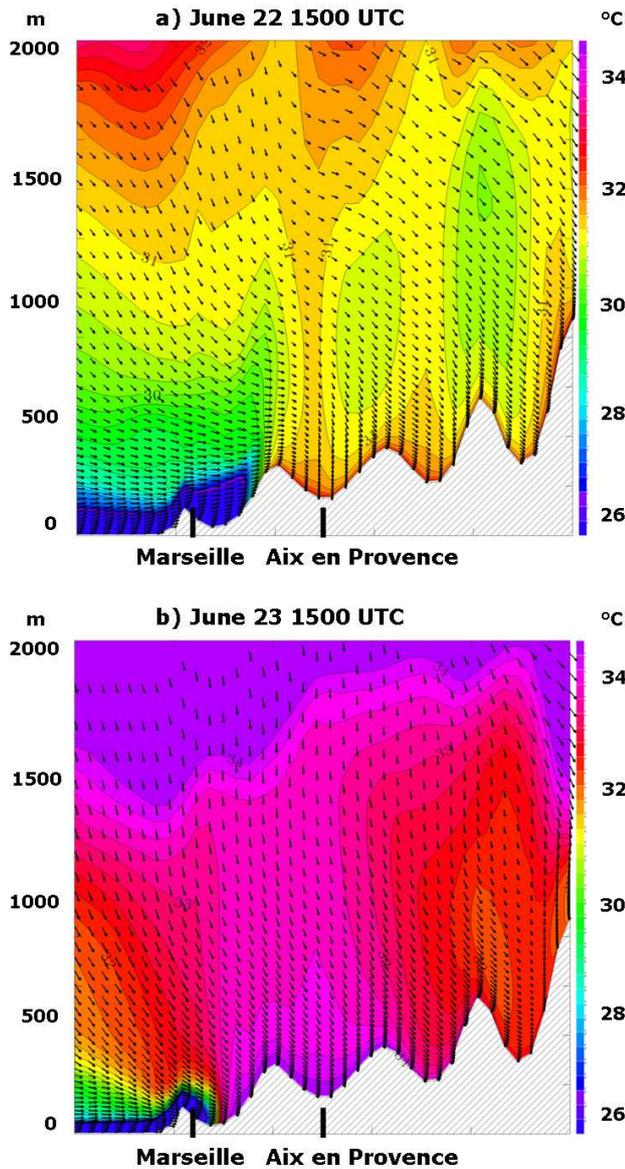
**Fig. 9.** Vertical section of potential temperature (color scale) and horizontal wind simulated by Meso-NH along an axis Marseille-Aix en Provence on 22 June at 15:00 UTC (a) and on 23 June at 15:00 UTC (b). The location of the cross section is shown in Fig. 16b.
