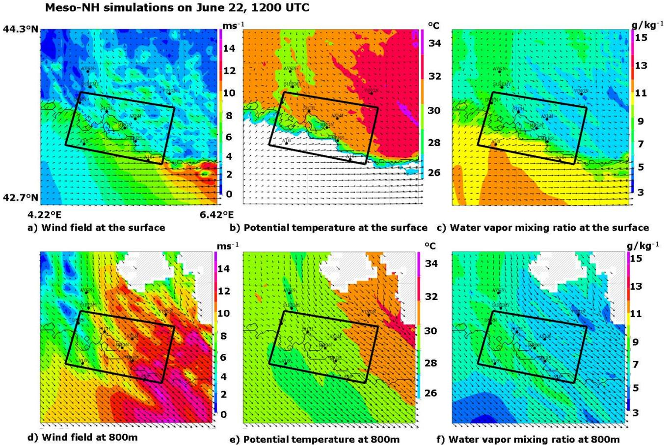
**Fig. 3.** Maps of wind speed and direction ( $\text{m s}^{-1}$ ), potential temperature ( $^{\circ}\text{C}$ ) and water mixing ratio ( $\text{g kg}^{-1}$ ) at the surface (top) and at a 800-m height (bottom) simulated on 22 June at 12:00 UTC with Meso-NH. The quadrilatere delimits the area flown over by the aircraft.
