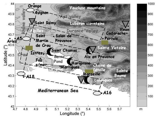
**Fig. 1.** Map of the various instrumented sites and horizontal track of the flights performed by the aircraft during the ESCOMPTE field experiment. Ellipses represent aircraft sounding locations. Triangles indicate radio-sounding sites and black half-moons correspond to the location of UHF wind profilers. Grey rectangles indicate the surface flux stations. Names of town, mountains and valleys are written in black, white and grey, respectively.
