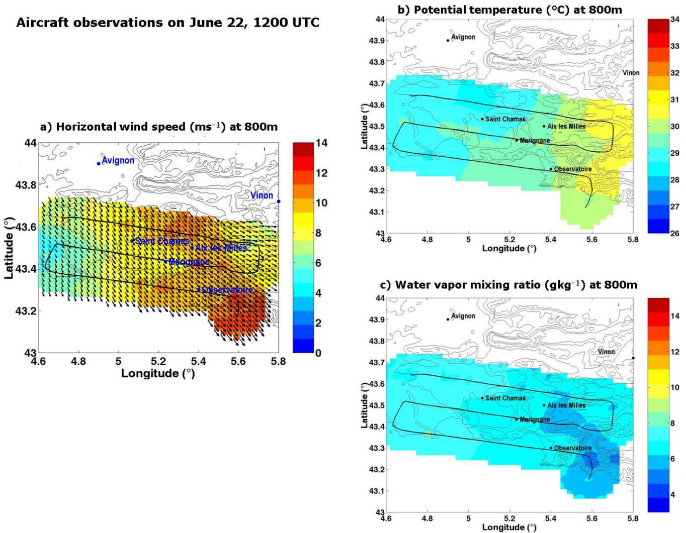
**Fig. 4.** Fields of wind speed (a), potential temperature (b) and water vapour mixing ratio (c) retrieved from aircraft measurements at 800 m on 22 June between 11:00 UTC and 12:30 UTC. The flight track is represented with a black solid line.
