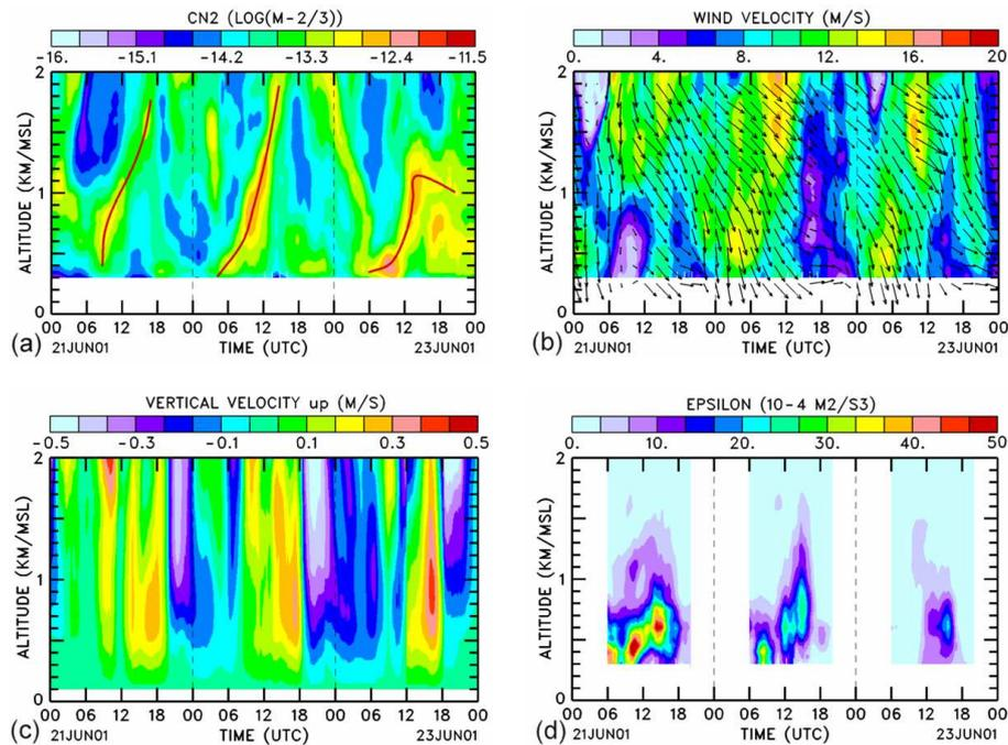
**Fig. 8.** Height-time cross sections of the structure constant  $Cn^2$  ( $m^{-2/3}$ ) (a), horizontal wind ( $m s^{-1}$ ) (b), vertical velocity ( $m s^{-1}$ ) (c) and dissipation rate of turbulent kinetic energy ( $10^{-4} m^2 s^{-3}$ ) measured with the UHF wind profiler in Saint Chamas during the Mistral episode (J21 to J23). The red solid line in panel (a) represents the ABL top height.
