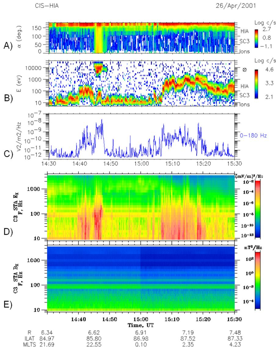
**Fig. 15.** 26 April 2001. From top to bottom: (A) Ion pitch-angle distribution from HIA for all ions. (B) Energy-time spectrogram from HIA for all ions. (C) Electric field spectral density from 0 to 180 Hz from the STAFF instrument. (D) Frequency-time spectrogram for electric field waves from STAFF in the frequency range from 10 to 3000 Hz. (E) Frequency-time spectrogram for magnetic field waves from STAFF in the frequency range from 10 to 3000 Hz.
