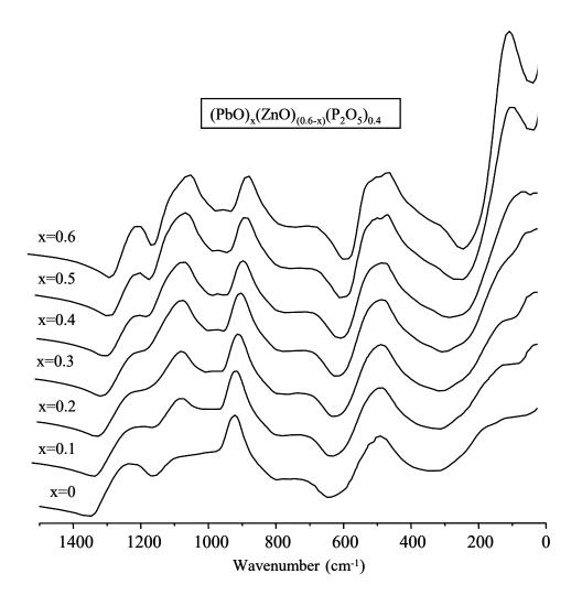
**Figure 1:** IR reflection spectra of (PbO)<sub>x</sub>(ZnO)<sub>(0.6-x)</sub>(P<sub>2</sub>O<sub>5</sub>)<sub>0.4</sub> glasses.
