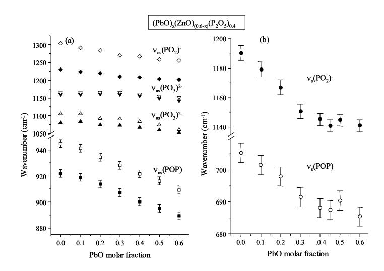
**Figure 3**: Lead content dependence of the  $v_{as}(PO_2)^-$ ,  $v_{as}(PO_3)^{2-}$ ,  $v_{as}(POP)$  deduced from IR spectra (TO mode are in plain symbol and LO in open symbol) (a) and  $v_s(PO_2)^-$ ,  $v_s(POP)$  deduced from Raman spectra (b) in the  $(PbO)_x(ZnO)_{(0.6-x)}(P_2O_5)_{0.4}$  glasses.
