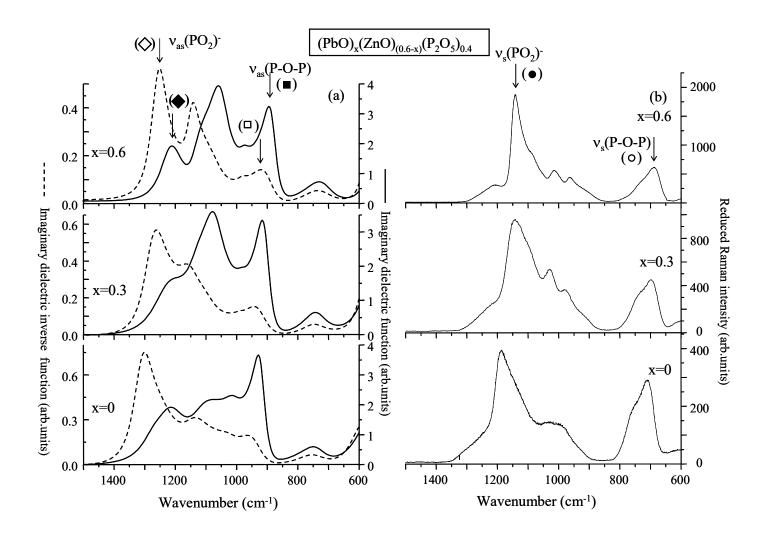
**Figure 2:** Imaginary parts of the dielectric (—) and the inverse dielectric (---) functions (a) and reduced Raman spectra (b) of the  $(PbO)_x(ZnO)_{(0.6-x)}(P_2O_5)_{0.4}$  glasses.
