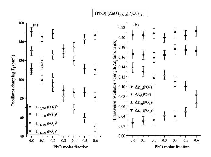
**Figure 4:** Lead content dependence of the  $\Gamma_j$  (a) and  $\Delta \varepsilon_j$  (b) deduced from IR simulation spectra in the (PbO)<sub>x</sub>(ZnO)<sub>(0.6-x)</sub>(P<sub>2</sub>O<sub>5</sub>)<sub>0.4</sub> glasses.
