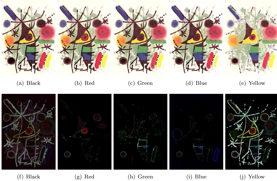
Fig. 6. Influence of the reference color on the graph ordering for an erosion.
