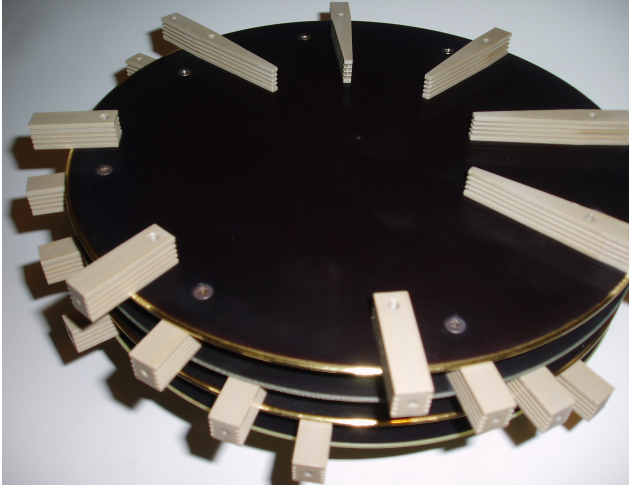
Fig. 5. Part of the HV deflection/collimation system which consists of circular plates and supporting PEEK insulators/spokes (the top plate is removed).
