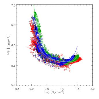
**Fig. 3.** A scatter plot of the perpendicular electron temperature against the electron density derived from PEACE on-board moments calculated by the HEEA sensor. A fourth order polynomial curve was fitted to the points from each spacecraft (shown). Each data point was projected onto the curve corresponding to the same spacecraft, and the distance along the curve to each projected point was converted to the transition parameter by normalising to extreme values.
