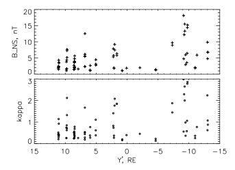
**Fig. 11.** Distributions of the median magnetic field in the neutral sheet  $B_{NS}$  (upper panel) and the adiabaticity parameter  $\kappa$  (bottom panel) versus Y'.
