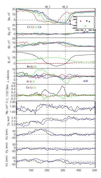
**Fig. 1.** 500 s of Cluster data from  $\sim$ 15:25 UT, 12 August 2001. From top to bottom:  $B_X$ ,  $B_Y$ ,  $B_Z$  from all four spacecraft; three components of **B** at the Cluster barycentre; three components of the calculated current density **j**; X-,Y-, and Z-components of the magnetic field curvature vector  $\mathbf{C}=(\mathbf{b}\cdot\nabla)\mathbf{b}$ ;  $\mathbf{H}^+$  density, pressure and bulk velocity (three components) from Cluster 1 and 4.
