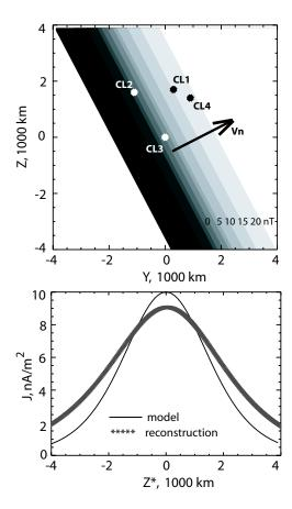
**Fig. A1.** Upper panel: Model of flapping motion of 1-D current sheet, magnetic field intensity is gray-scale coded. Bottom panel: Model (solid line) and reconstructed (asterisks) profiles of current density.
