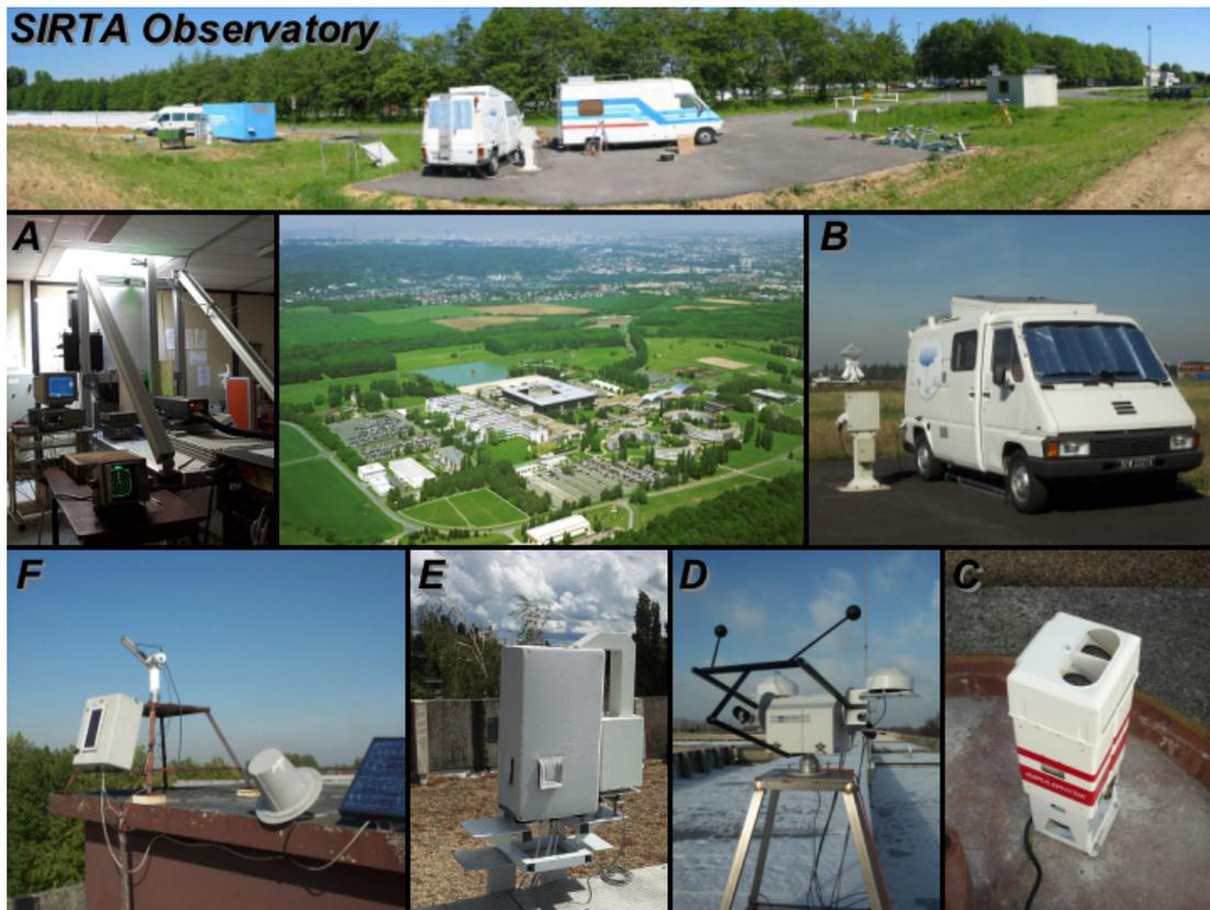
**Fig. 2.** Photographs the main components of the SIRTA observatory: overall view of the Ecole Polytechnique campus (center panel), measurement platforms (top panel), (A) LNA lidar, (B) RASTA radar, (C) ceilometer, (D) surface radiative flux station, (E) Drakkar MWR, and (F) Sun-photometer.
