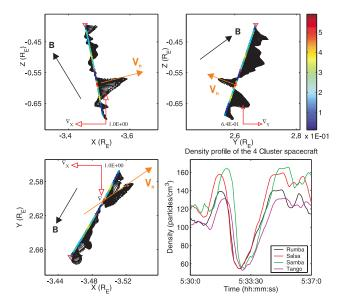
**Fig. 8.** Density gradient vector projections onto the XY, YZ, and XZ GSE planes for the density irregularity Z observed in the plasmasphere on 11 April 2002. B is the magnetic field and  $V_n$  is the normal boundary velocity of the inner edge of Z. The density of the four spacecraft is plotted as a function of time in the lower right panel.
