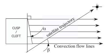
**Fig. 2.** Illustration of the satellite trajectory orthogonal to the plasma flow. The important parameters defining the uncertainty in a velocity dispersion analysis are the angles  $\alpha$  (flow – source angle) and  $\beta$  (spacecraft trajectory – flow angle).
