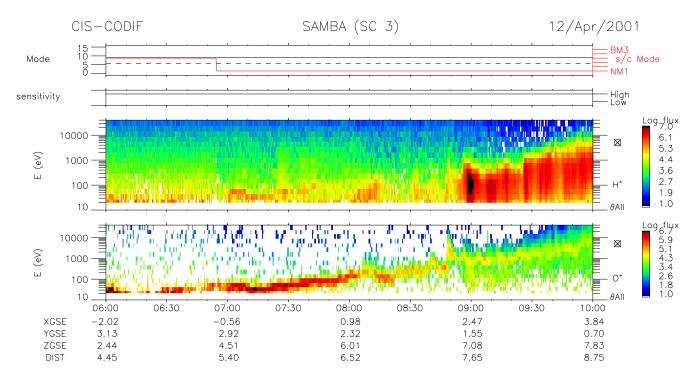
**Fig. 3.** Cluster spacecraft 3 (Samba) data from 12 April 2001. Panel 1 shows spacecraft mode, panel 2 instrument mode. Panels 3 and 4 show the H<sup>+</sup> and O<sup>+</sup> energy spectrograms, particle flux integrated over all directions.
